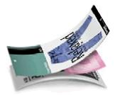
An RF-EAS security tag, sandwiched between the branding and tracking components, is invisible to the customer.
