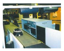
CHECKED BAGGAGE passes under RFID scanners at Northwest Airlines' Seattle-Tacoma facility. Any suspicious bag is tagged and pushed off this conveyor belt by diverters (seen in the middle of the photo) and transported to an explosive detection system. The view is through the second, failsafe set of RFID readers, looking upstream toward conveyors and deflector. Photo courtesy of SCS Corp.
