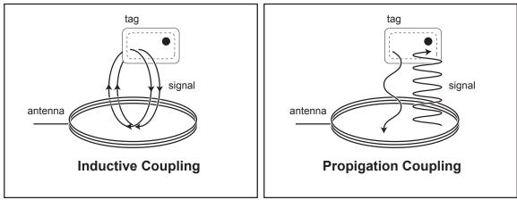
Tags and a reader communicate by wireless signal in a process known as *coupling*.
