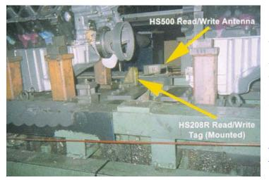
Ford Motor Co. is using RFID tags to streamline its Essex engine plant in Windsor, ON.
